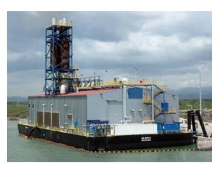
The Power Express 1020 is a barge MPGV with high mobility and maneuverability in tight spaces, and to carry it quickly and effectively to remote villages near the coast or a river supplying large amounts of energy with a minimal investment in mainland.
